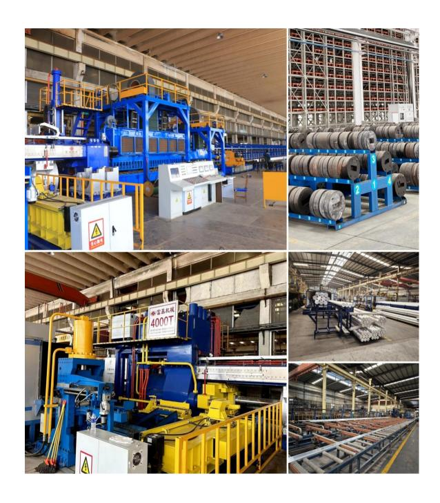
The factory can produce various large, medium, and small cross-section aluminum profiles, with mold cross-sections ranging from 10mm to 400mm, to meet customers' diverse customization needs.
