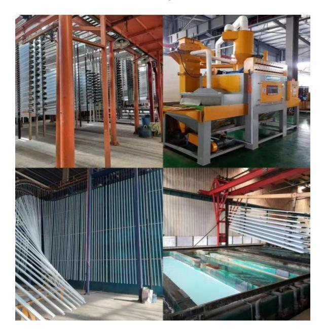
The common surface treatment methods for aluminum profiles are complete, including color anodizing (sandblasting, alkali sand, two acid, three acid, three acid, hard), electrophoresis, powder coating, fluorocarbon coating, wire drawing treatment, polishing, wood grain heat transfer printing, etc., which can meet various production needs and large-scale operations.
